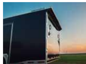
Rivetless side sheets on 4410
