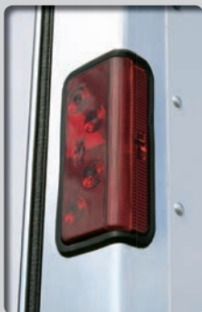
Wraparound Lights. Featherlite horse trailers are outfitted with stylish L.E.D. wraparound lights that give your trailer more visibility when traveling down the road. Plus, four stop/turn L.E.D. lights are standard on horse trailers.
