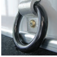
Rubber coated tie rings for a quieter, less stressful ride under mats.
