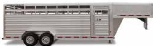
Model 8117. Model 8117 livestock trailer is designed after the popular Model 8127 and comes with an aluminum floor standard and 3" crossmembers on 12" centers. Model 8117 is available in 16', 20' and 24' lengths and is 6'7" wide.
