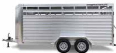
Model 8107. Bumper pull stock trailer with aerodyne nose. Available in standard or low-profile heights (5'3"). Length options are 12', 16' and 20'.
