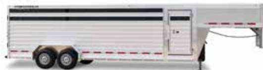
Model 8127. Gooseneck trailer Model 8127 is available in lengths ranging from 16' to 36' and comes with Featherlite's durable all-aluminum floor. Choose from an almost endless list of customization options. 7', 7'6" or 8' wide.
