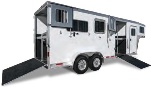
Model 9752. Straight load trailer features a 2+1 configuration with a rear ramp and side ramp. It includes a 24" walk through aluminum door and aluminum lined ceiling. Trailer is 6'7" wide, 7'6" tall and 22' long.
