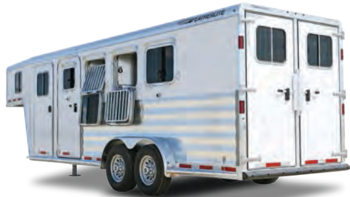
Model 8541. This slant load can be customized to hold 2 to 6 horses and offers many dressing room sizes. Model 8541 comes standard with white aluminum lining in the horse area and is available in widths of 7' or 7'6". Also available with living quarters.
