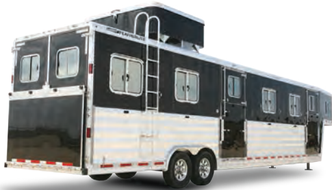
Model 9810. Model 9810 is a straight load 6-horse. It features a tack room and ramps on both sides of the trailer. Shown with many options including hay rack and black side sheets. 9-horse configuration optional!
