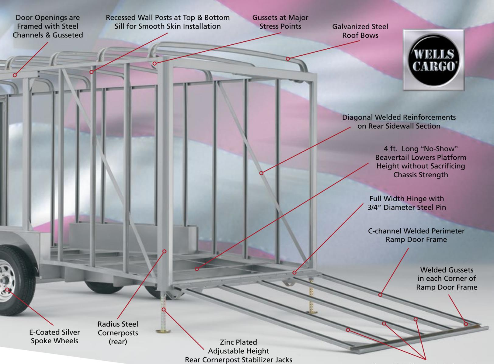
Door Openings are Framed with Steel Channels & Gusseted
