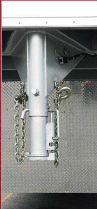
Standard AWG Hitch (2 5/16" Adjustable Height Ball Hitch)
