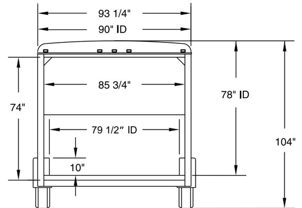
NOTE: The Tapered Nose Gooseneck is also available in the standard 93 1/4" body width.
