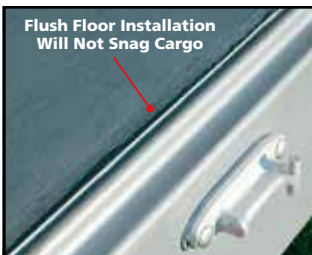
Recessed Z-Pan Seals Out Dust
