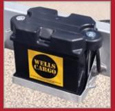
Breakaway System with Wet Cell Battery
