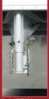
Standard AWG Hitch (2 <sup>5</sup>/<sub>16</sub>" Adjustable Height Ball Hitch)
