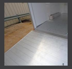
Rear ramp door with covered, continuous hinge
