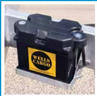
6 Breakaway System with Wet Cell Battery
