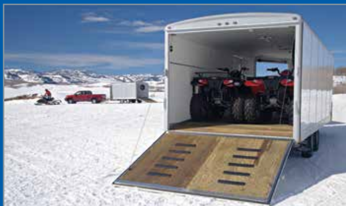
92"W Rear Ramp Door w/ Spring Assist (optional Traction Blocks)
