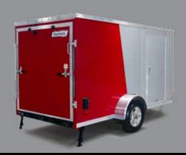
Haulmark's goal when designing the new V-Series CARGO trailer was to set the industry benchmark for durability & performance for years to come. High-strength low-alloy (HSLA) steel, patent-pending roll-formed components and 100% dipped coated frame for ultimate corrosion resistance
